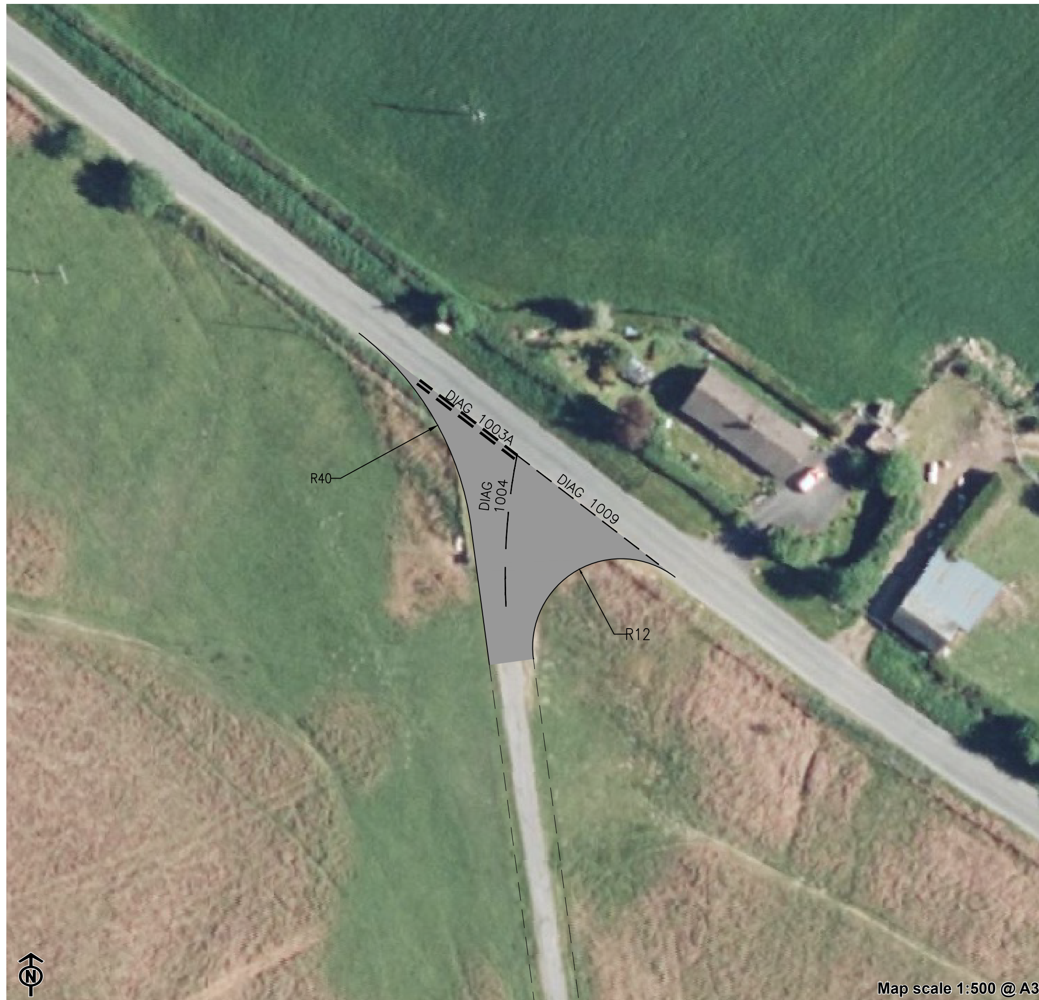
Figure 4.9a: Site Access Arrangement
